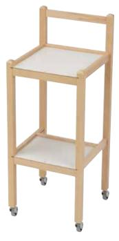
The top shelf is at the ideal height for sliding a plate on from the worktop and the lower shelf has a cutaway for the user's legs. The castors have rubber tyres for easy manoeuvring across a range of floors.
