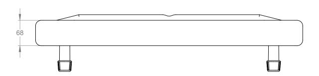
FITS A UK STANDARD BATH OF 700mm OVERALL WIDTH MAXIMUM PILLAR SPAN = 630mm MINIMUM PILLAR SPAN = 440mm
